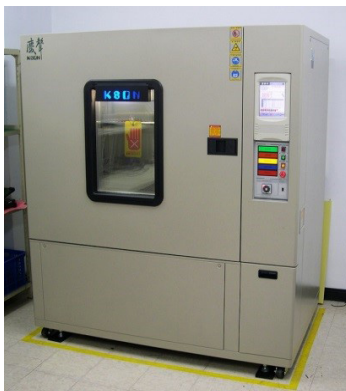
High / Low Temp and humidity Chamber (-50°C to 150°C)
