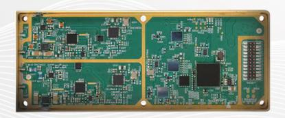
Feature Specification 100MHz to 3GHz Frequency Range 100MHz to 3GHz Frequency Hopping Range Data Bandwidth 1Mbps Bandwidth Ethernet Frames + Video Stream **Data Transmission** Data Terminal Interface ENET, USB Input Power 10-28VDC RF Input Power Active Gain up to 1W AES-256 Encryption -20 C to 55 C Operating Temp Ingress Protection Dimensions Embedded Module 65mm x 60mm x 25mm Tactical Module 65mm x 60mm x 40mm Embedded Module 130g Tactical Module
