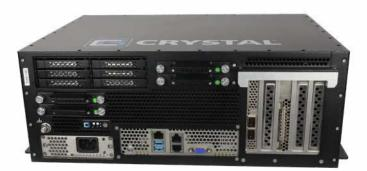
**Field-tested, fail-safe and long-life performance in extreme conditions.** This feature-rich embedded computer system is powerful, compact, and rugged. Designed for applications requiring a small footprint with GPU capabilities, the RE1739 is ideal for signal processing and autonomous vehicle sensor processing and inference. The integrated DC power supply is designed for low-voltage noisy vehicular applications.
